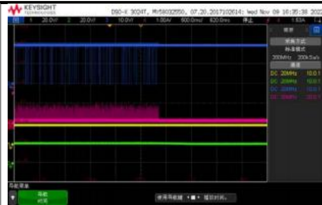
CH1: VIN CH2:VOUT CH3:SW CH4:IL Vin=20V Vout=20V Shut Down waveform through EN, Iout =0A
