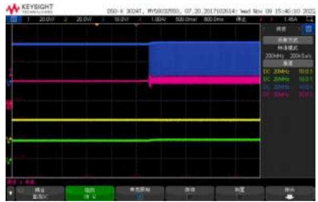
CH1: VIN CH2:VOUT CH3:SW CH4:IL Vin=20V Vout=20V Start up waveform through EN, Iout =1A
