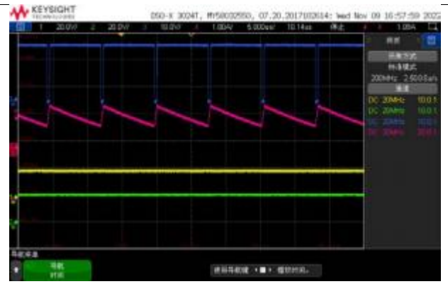
CH1: VIN CH2:VOUT CH3:SW CH4:IL Vin=20V Vout=20V Steady State waveform Iout =1A
