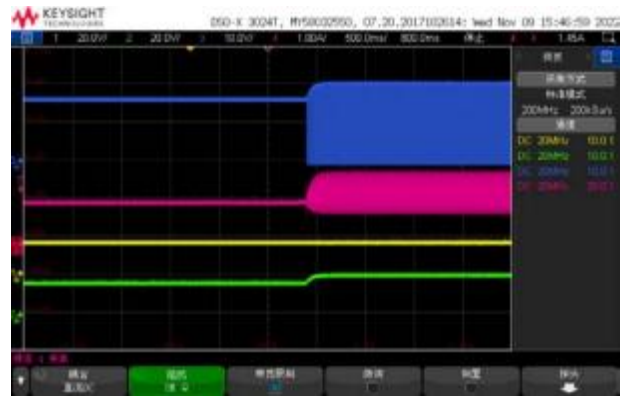
CH1: VIN CH2:VOUT CH3:SW CH4:IL Vin=16.8V Vout=20V Start up waveform through EN, Iout =1A
