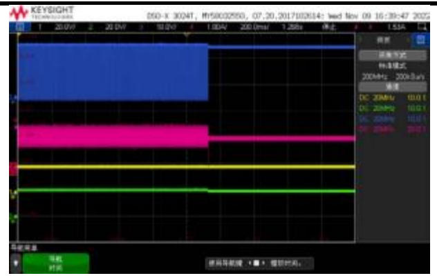
CH1: VIN CH2:VOUT CH3:SW CH4:IL Vin=20V Vout=20V Shut Down waveform through EN, Iout =1A
