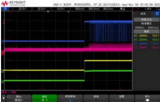
CH1: VIN CH2:VOUT CH3:SW CH4:IL Vin=20V Vout=20V Start up waveform through EN, Iout =0A
