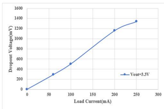
Figure10 Dropout Voltage vs Load Current
