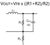
Vref is the internal reference voltage of DP31240B/FB, 0.8V.
