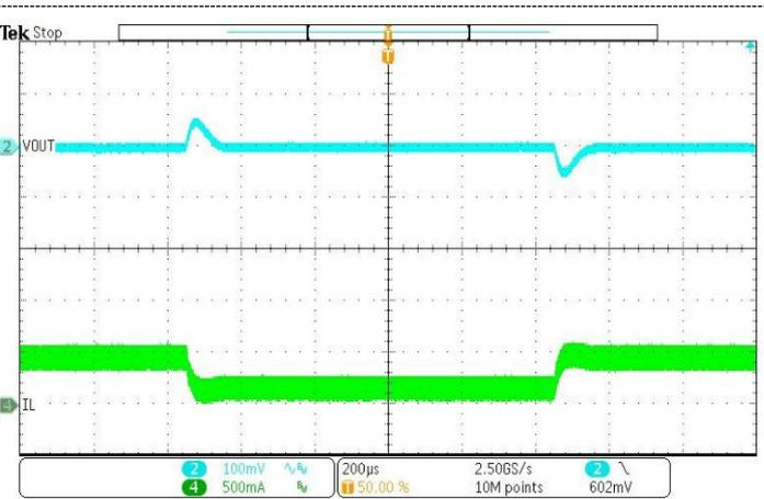
Load Step 0.15 to 0.5A, 1A/us Slew rate
