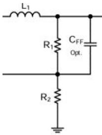
Vref is the internal reference voltage of DP31240B/FB, 0.8V.
